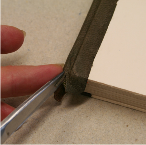
FIGURE 213 The making of the next cut at the other joint, so that the next turn-in can be made. After this, the remaining extending part of the spine leather forms the tab.
