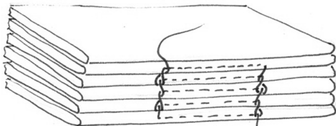
FIGURE 25 A link-stitch on two stations. The thread exits one gathering in order to pass to the next, it is then taken behind the point of exit in the previous gathering, thus forming a chain of linkages.
