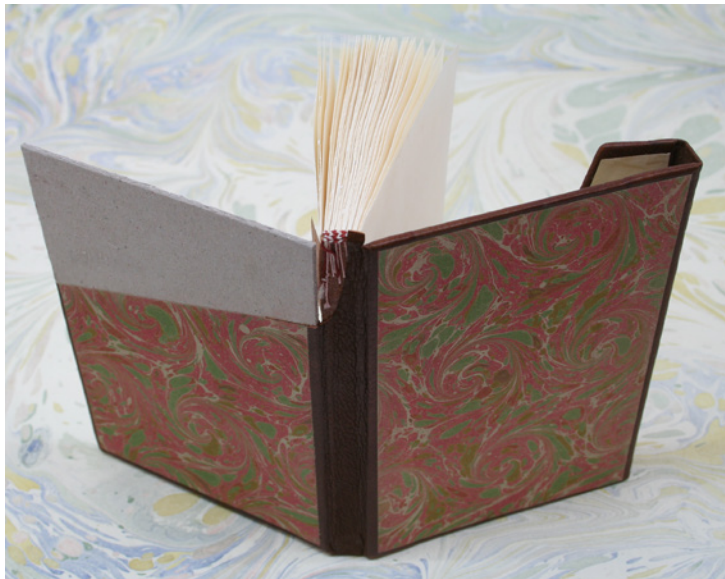
FIGURE 208 A see-through model with a leather spine-lining. The binding has a partial leather covering with leather strips on all board edges.
