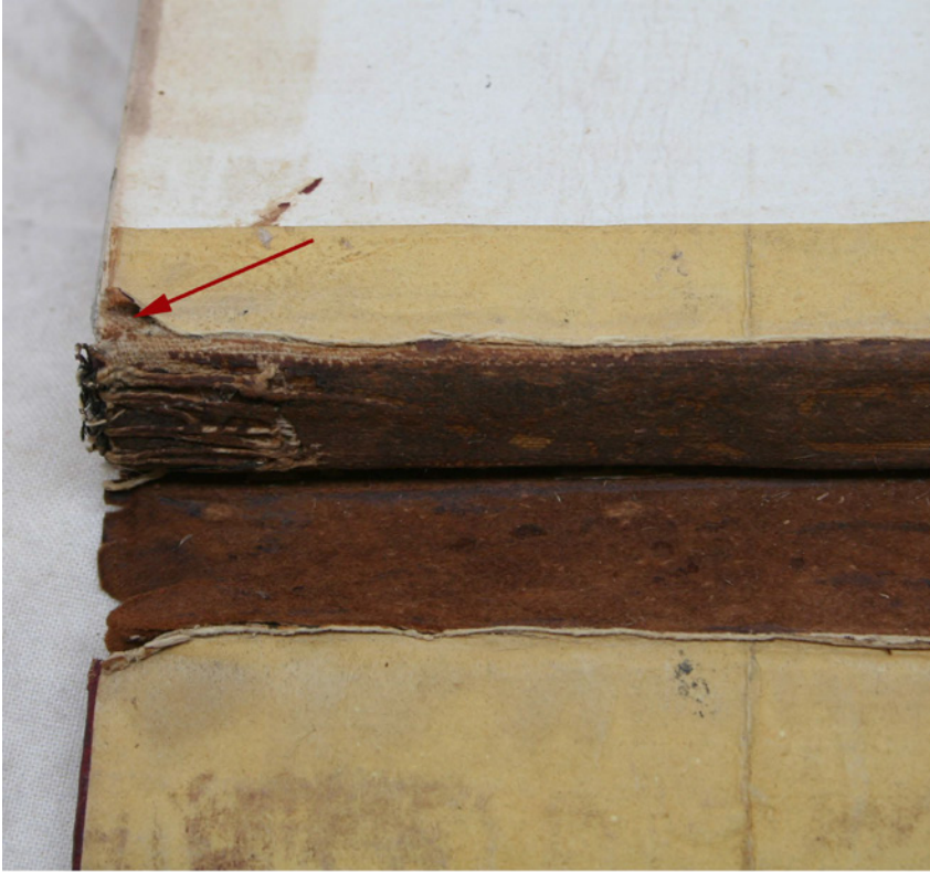
FIGURE 62 Or. 2686 (1844) . The extension of the cloth lining was adhered onto the outer leaves of the textblock; it did not function in the board attachment structure. Now that the adhesive with which the leather was pasted onto the textblock spine has lost its strength, the paper joint has split. The remaining stub covers the cloth pasted onto the textblock's outer leaf.
