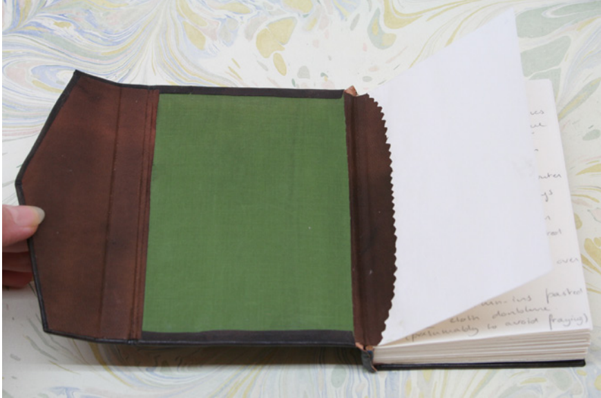
FIGURE 204 A model of a full leather binding with cloth doublures on the boards, a leather doublure on the flaps, and an additional leather inner joint. The leather turn-ins overlap the cloth.
