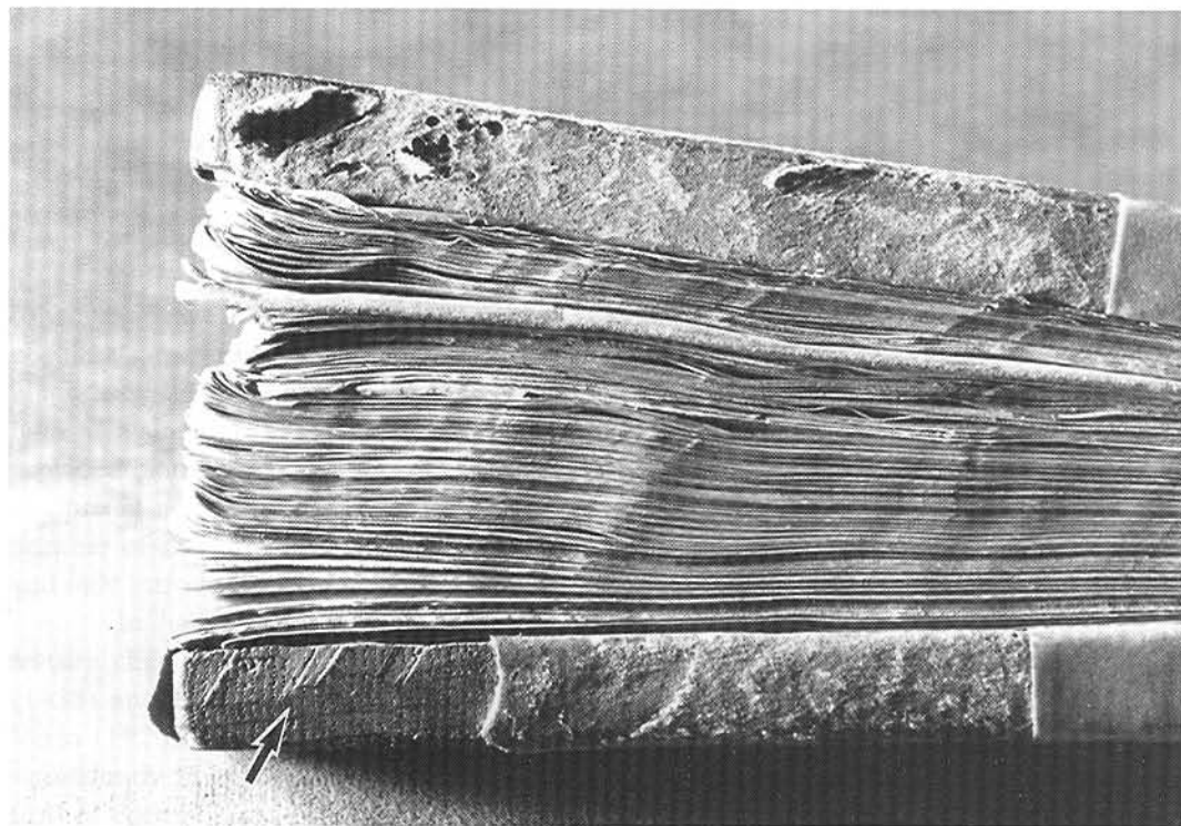
Figure 7.20 Head edge of SG Cod. 459 (s. x) with oblique score marks from the drawknife. Marks on the lower board (arrow) seem to run from the bookblock onto the edge; perpendicular year rings indicate that the board was cut on the quarter (from Szirmai 1995).
