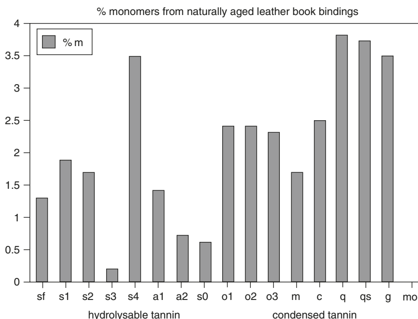
Figure 5.8 Comparison of analysis of % monomers in extracted tannins from different species used in the British long-term tests in book bindings from books placed in the British Library in 1932. The ageing environments were the same for all tannins. Raw data from Larsen (2000). sf = sulphited sumac; s = sumac; a = acacia; n = new; o = oak; m = mimosa; q = quebracho; g = gambier; %m = % monomers in extractable tannin.
