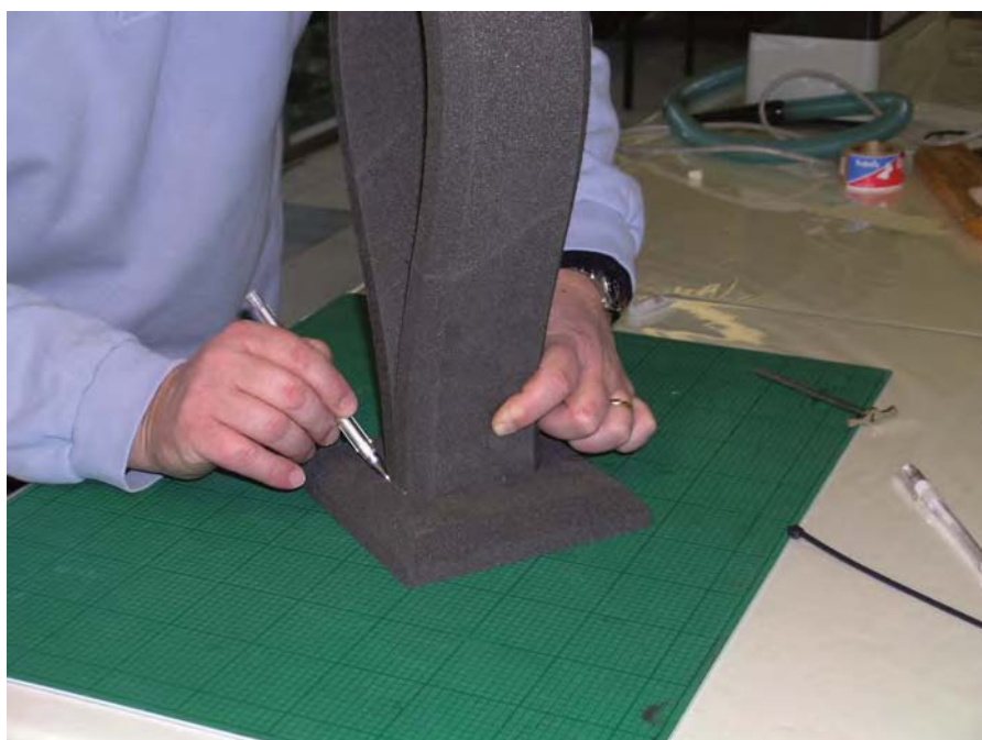
Figure 23.48 The mount is folded over and placed on the centre of the base so that the profile can be transferred onto the base and the location hole cut out.
