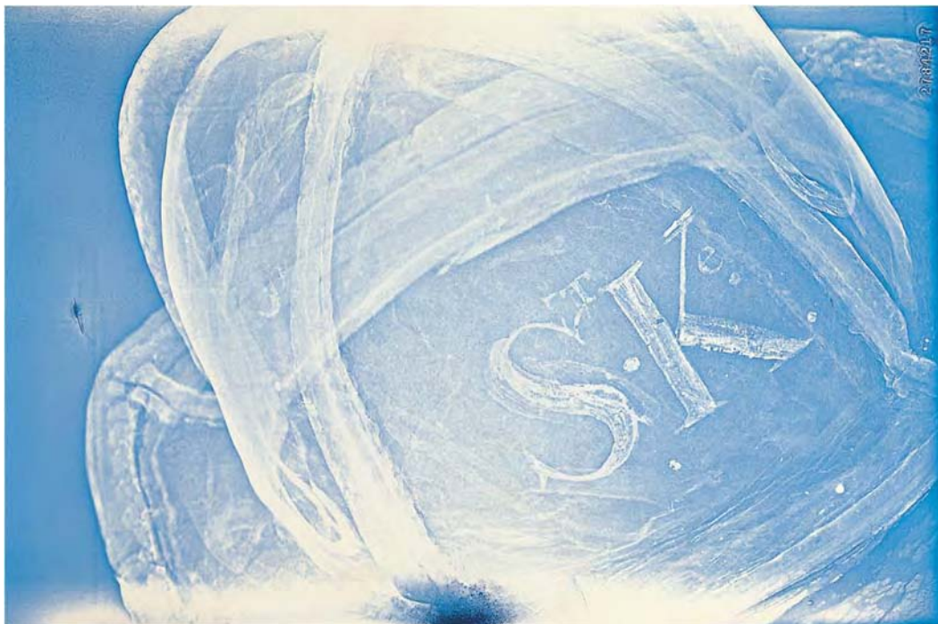
Figure 10.4 Xeroradiograph of the helmet showing construction of helmet and lead white lettering on original surface of the helmet. (Courtesy Barry Knight, Science Conservation Department, English Heritage)
