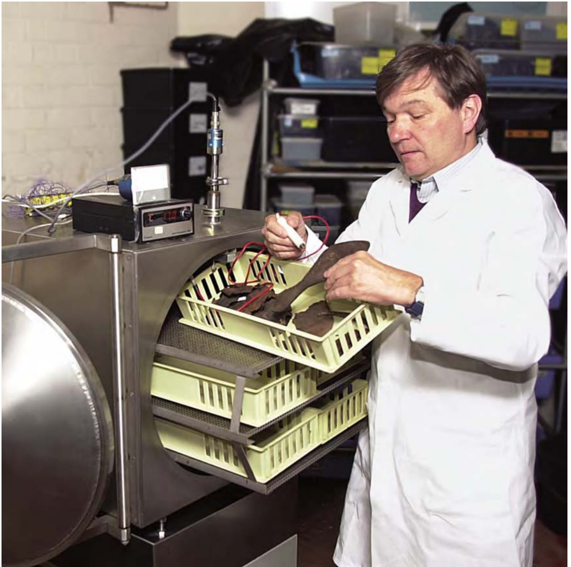
Figure 22.2 Preparing a load for accelerated freeze-drying: a temperature probe is being inserted into a sample waterlogged leather piece. (Courtesy York Archaeology Trust)
