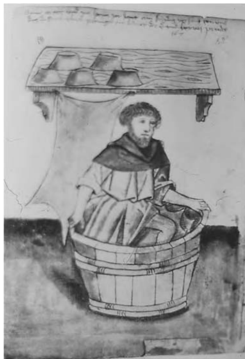
Figure 7.9 Working the tawing mixture into the skins mechanically in the foot-tubbing process.
