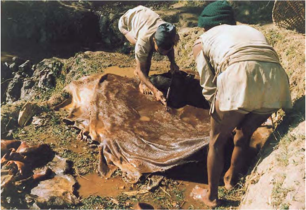
Figure 8.1 Sarkis are Nepal's traditional leatherworking caste. This hide, which has been tanned in a crude pit sunk in the ground, is being cut into sides before further simple processing. The stigma attached to this low-caste occupation caused a decline in rural tanning and leather product manufacture until the United Mission to Nepal established the Village Leather Training Association to encourage its revival. These simple methods reflect today what rural tanning and shoemaking would have been like in Europe in medieval times.
