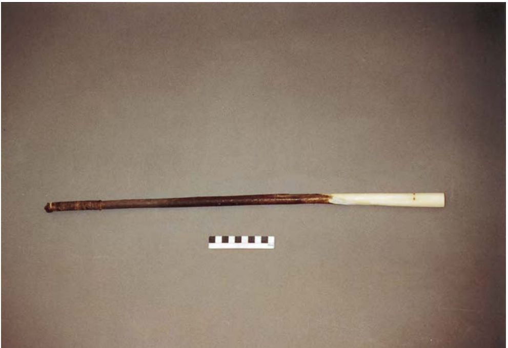
Figure 23.5 New timber spliced onto handle.
