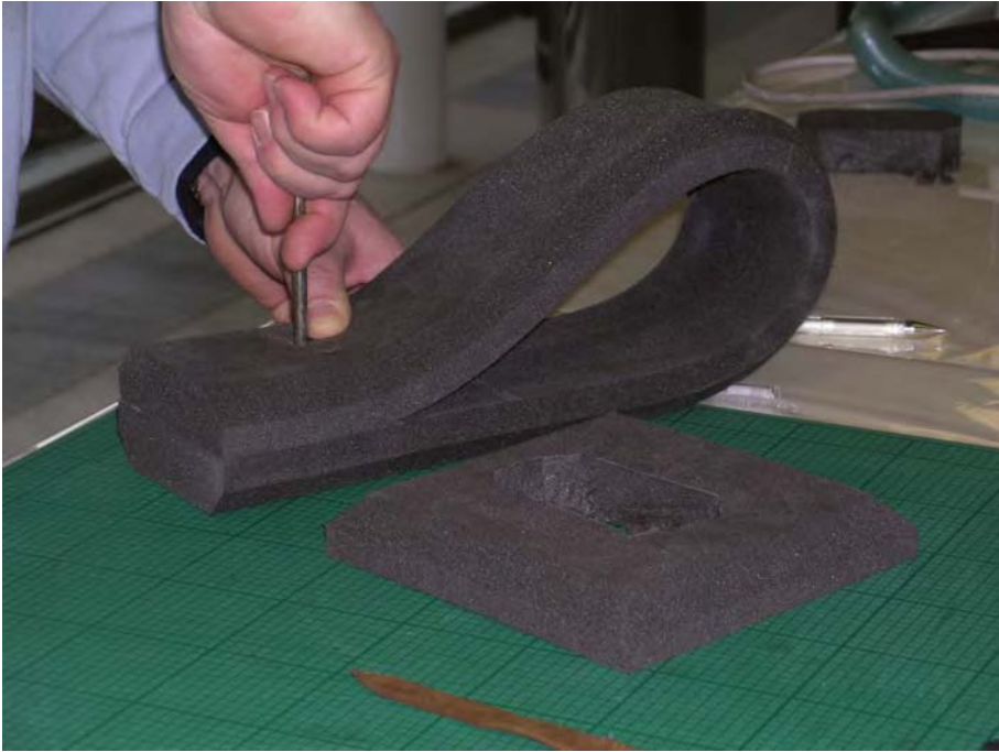
Figure 23.49 Two holes are punched through the mount near the base.
