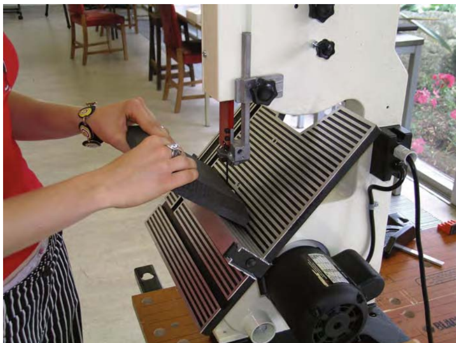
Figure 23.47 The Plastazote is cut to shape and size on a small hobby band saw. This is not essential and can be done with a knife. The chamfered edge on the base is for aesthetic reasons but is not essential. The chamfered edge of the main support softens the edge where it comes into contact with the helmet.
